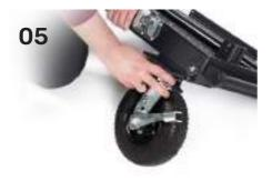
Lift one side of the lower platform by approximately 25 cm and slide the swivel wheel fork into the wheel slot located close to the edge with the handle. Secure the wheel against sliding out by using the lock on the upper side of the lower platform above the wheel slots – the lock must descend visibly, meaning that it is fully locked. Also ensure that the wheel fork has been completely slid into the wheel slot (the upper plate of the fork has been entered into the slot completely).
