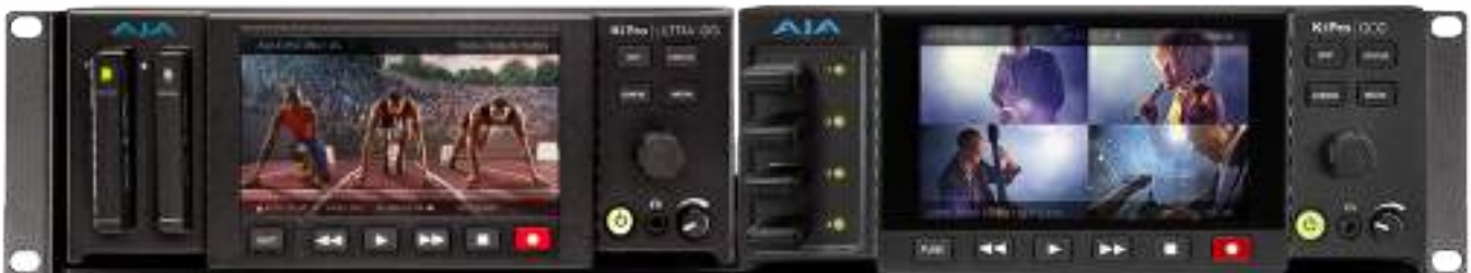
Figure 9. Ki Pro GO2 mounted in Rackmount Shelf with a Ki Pro Ultra 12G.
