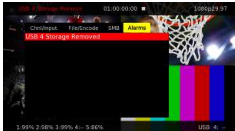
Figure 17. Status Menu, Alarms Tab.
