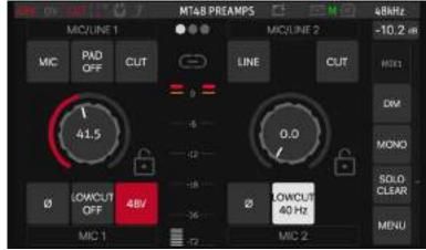
Each preamp has a gain knob as well as several additional functions.
