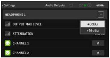
You can even reverse the signal polarity for each ear cup on each headphone output. Reversing one earcup (temporarily) can be useful to check for wiring mistakes. Reversing both cups is a useful option for some older headphones that came with reversed polarity. Correct polarity is crucial for singers in front of a microphone, so the electric path is in phase with acoustic path (air, skull bones).
