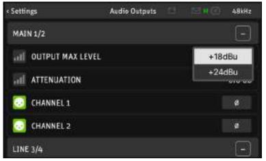
+24 dBu results in slightly better signal-to-noise but may be too hot for some equipment. When directly connecting your (active) studio loudspeakers, the lower signal level +18 dBu may be useful to prevent ear blasting SPLs. If needed, you can dial in additional signal attenuation.
