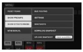
Pressing the MENU button in the upper left-hand corner, you can choose to display the preamp controls in all preamp-equipped input channels and/or the Effects knobs (EQ and DYN buttons and REV level). The latter will also give you edit panels in the left-hand side, if you click on an EQ or DYN button or open REV edit.
