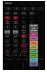
Please note that when you press on a rotary control (e.g. preamp gain or REV level) to change its value, a panel opens with a slider. This is to facilitate using the Web Control from a touch-screen device, e.g. a tablet computer.
