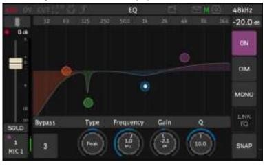
Please note: The EQ Gain and Frequency can be adjusted with touch movement on TFT. Make sure you update to the latest Firmware to benefit from such feature.
