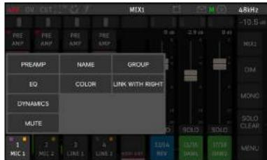
The entries PREAMP, EQ, and DYNAMICS allow you to access the respective pages without switching to the Alternate Mix View.
