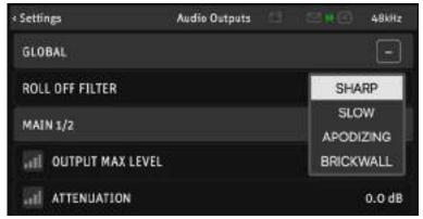
**Sharp** (default setting): Offers a flat frequency response with an attenuation of 3 dB at 0.484 x FS (23.2 kHz @48k), which has the tradeoff of 35 samples latency.
