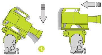
If the camera tilts forward (points downwards), then the camera must be moved towards the rear of the head (aft).
