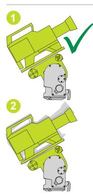
Tilt the camera approx. 45° upward and release it. If the camera stays in the same position when released, the camera is correctly balanced with the C of G on the tilt axis.
