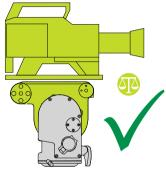
If the camera cradle stops in a horizontal position (camera pointing directly forward), the balance is correct.
