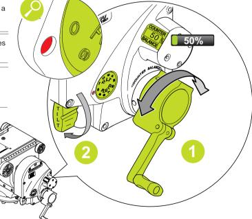
Hold and steady the camera, then disengage the tilt lock and observe how it moves and where it stops.
