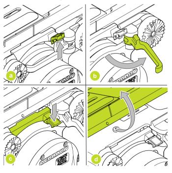
2. Attach the mounting plate securely to the bottom of the camera in the desired position.
