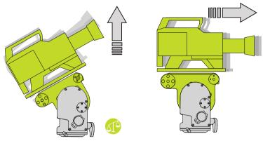
If the camera tilts backwards (points upward), then the camera must be moved towards the front of the head (fore).
