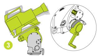
If the camera keeps falling back towards the vertical position when released, increase the counterbalance.
