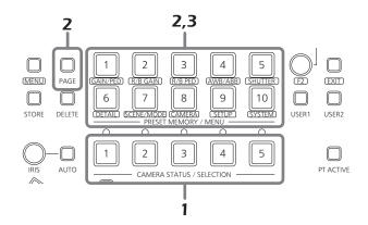
When the preset memory data is executed, the preset number is displayed on the right side of the top level of the LCD panel.
