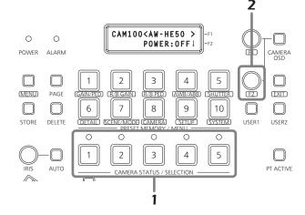
Turning off the power of a multiple number of cameras
