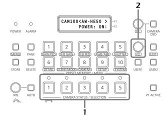
Turning the power of the cameras on simultaneously as the unit's power is turned on
