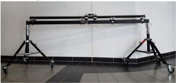
Mount the wheels and use not only the brake on the wheel but also angle the wheels towards the legs for utmost stability (right picture below)!
