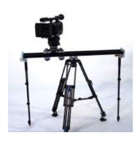
2. Mount the 2 Monopods underneath the Mini Sleepers (3/8" thread) at each end of the track. See that the Monopods really touch the ground by pressing up the Monopods against the track so that there is some tension on them.
