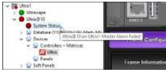
Figure 93 Example of a Master Alarm Message
