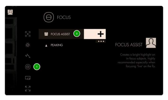
**Focus Assist** will paint a **highlight** around areas it determines to be in focus based on small/harsh changes in contrast.
