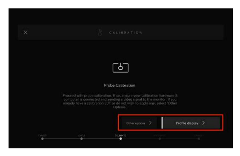
6. Position your probe against the monitor's screen according to the manufacturer's recommendations. Tap **Done** to begin the calibration process. You will then be prompted to browse for and apply an LUT or to skip this step.
