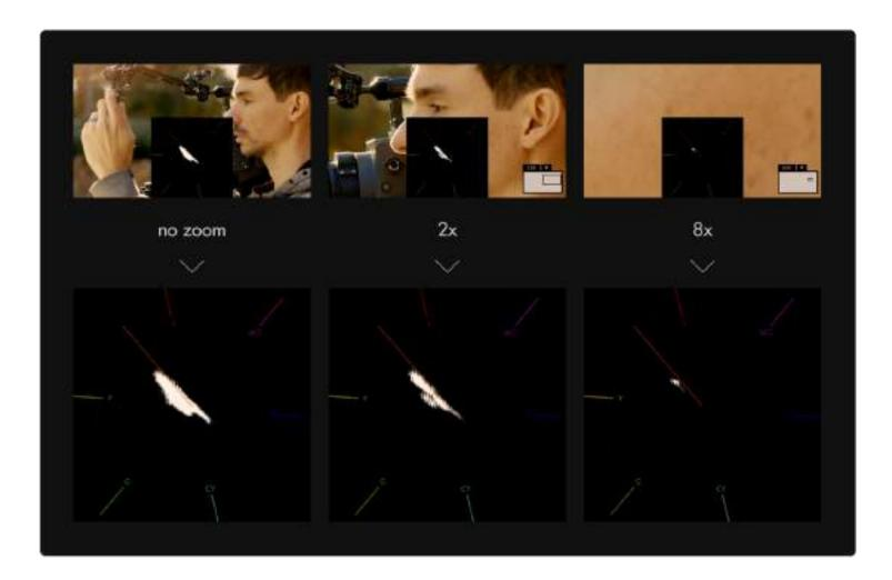
Zooming into an area consisting of **only** skin tones reveals the **exact hue** in which they plot - the result is **slightly** toward the **yellow** side - this is the result of a golden reflector which was used to bounce light onto the face. If we had used a silver reflector, the facial tones would rest precisely on the **skin tone line**.
