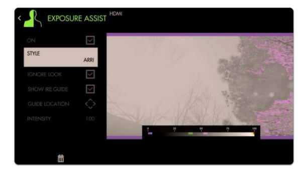
Even though the **sun** area is **clearly clipping**, the Arri false color scale doesn't pick it up - **we need to fix this for an accurate reading**.
