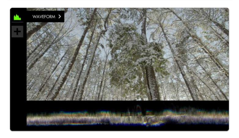
I have already added a <u>Waveform</u> to an empty page and adjusted its **height** from **50** down to **25** to make a bit more room for the image, but it is still **covering a portion of the picture** which we can address with **Scale & Position**.
