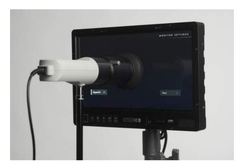
Follow the DisplayCal instructions, making sure that you have the correct monitor and probe selected. Also make sure that your calibration settings match the calibration target. We are not affiliated with DisplayCal so please refer to the documentation and support from DisplayCal for operating the software.
