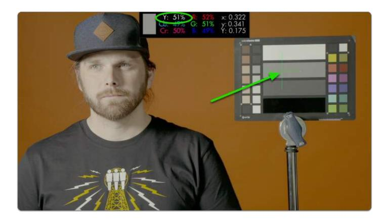
This particular color chip has been designed to read as 'middle grey'. Look for the 'Y' (luma/brightness) percentage and roll exposure until it reads **near 50**%.
