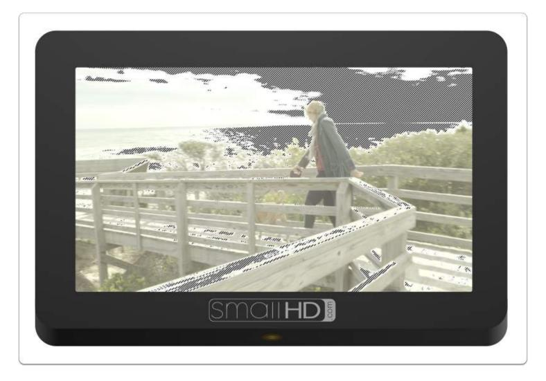
Zebra is essentially a simplified version of Exposure Assist which allows the specific 'painting' of areas depending on brightness value but is less destructive to the underlying image — it is however limited to painting one value range at a time, though up to two Zebra tools can be activated simultaneously. Click to learn more about the Zebra tool.
