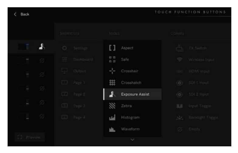
Notable configurations for Touch Function Buttons include Backlight Toggle, Backlight Custom, Input Select, and 4K TX Switch. Having different inputs on Touch Function Buttons allows the user to quickly switch sources, without having to navigate to the Monitor Settings menu.
