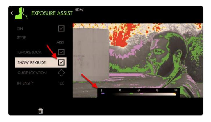
Exposure values near the **50**% mark on the scale will generally provide the most **natural result** on **human skin**. With the **Arri scale** this means the **pink** and **green** bands provide a great guide as the **upper** and **lower** range for exposing faces.
