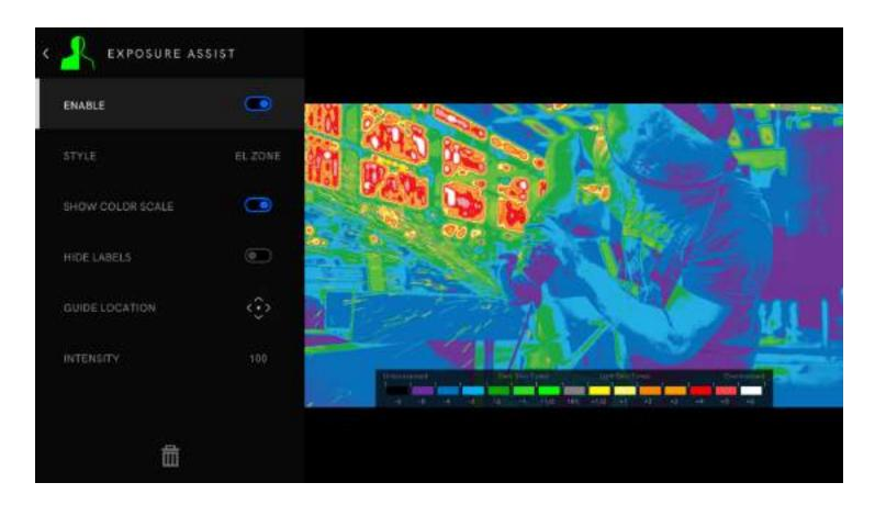
EL Zone is a stop-based exposure map tool—developed in collaboration with legendary cinematographer Ed Lachman, ASC that works like a virtual spot meter, replacing IRE exposure values with stops. Sensor data from the camera provides a reference point, and a false color represents each stop above and below 18% gray, allowing for easier, more intuitive on-set communication.
