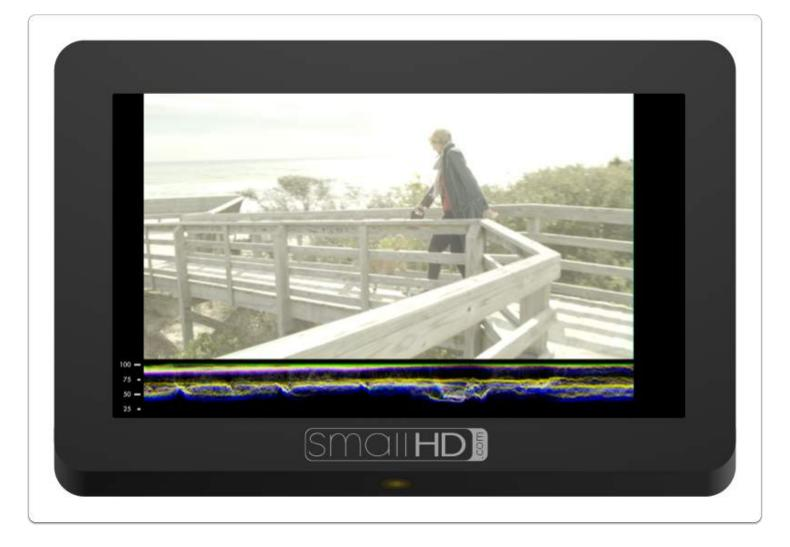
Waveform plots the value of the entire image onto a graph that physically matches it from left-to-right, meaning if you see an area that's too bright on the left side of the image, it will create a 'peak' on the left side of the waveform graph. It also has other benefits by way of RGB & RGB Parade modes. Click to learn more about the Waveform.
