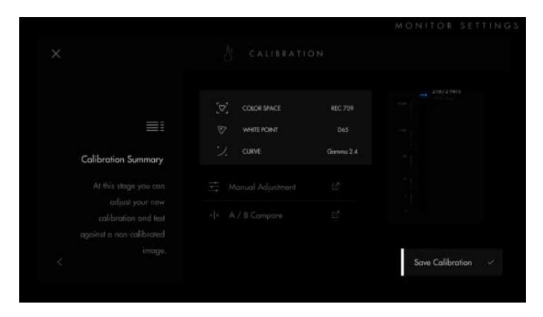
Your calibration will show up as Custom Calibration in the Calibration settings. You can toggle between Custom Calibration and Factory Calibration at any time.
