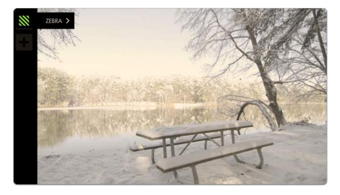
Because our camera **places its overexposure limit below 100%** or 100 IRE (quite common when shooting in log/flat gammas) **we need to adjust the minimum IRE** until the Zebra is activated.
