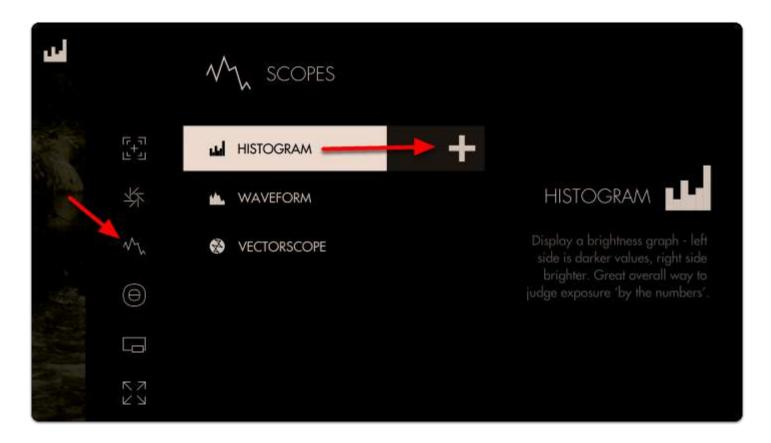
A graph appears in the top-right of the image. It will default to LUMA values (Overall Exposure). Histograms read Shadow levels on the left and Highlights on the right. The weight of the curve will tell you where your exposure values are falling along that scale.
