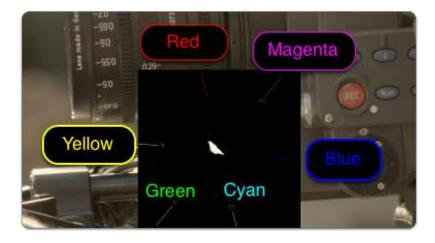
If we **apply a LUT** to this page, the Vectorscope reacts by **expanding** its plotted area. The scope confirms that we are viewing a more heavily saturated image after applying the look.
