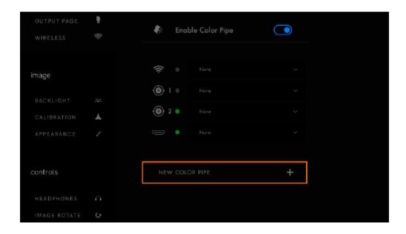
3. By default, the new Color Pipe standard is set to REC 709. Tap the scroll-down icon to make changes.
