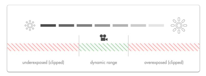
Adjusting **exposure** will shift the **dynamic range** to capture brighter or darker detail in order to accommodate the most important aspects of the image. Anything outside the **dynamic range** gets **clipped**, meaning a badly placed exposure is **wasting the camera's potential**.
