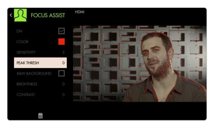
Bringing **Peak Threshold** up to around 30 does a better job of causing **only in-focus areas to activate the filter** but this is ultimately a balance that may need tweaking depending on the camera/shot.
