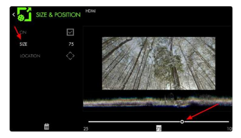
Now move the image to the top of the frame by selecting **LOCATION** and pressing **up on the joystick** or **tapping the top portion of the image**. This leaves us with an unobstructed view of the **Waveform**.
