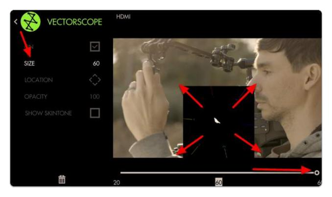
You can adjust the **SIZE** of the graph for better visibility. At this stage feel free to use <u>Size & Position</u> or <u>Crop & Scale</u> to <u>arrange</u> the image and scope so that they **don't overlap**.
