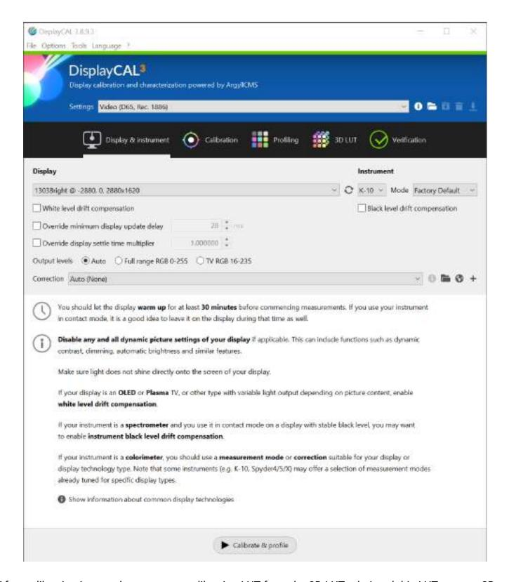
After calibration is complete, create a calibration LUT from the 3D LUT tab. Load this LUT onto an SD card and insert it into your monitor.
