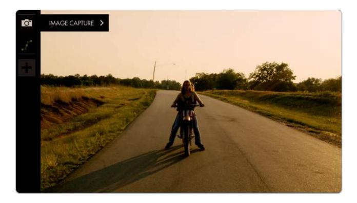
A grey snapshot overlay will appear; click the joystick or tap the screen and the overlay turns green, indicating a snapshot has been taken. The screen will also appear to flicker.
