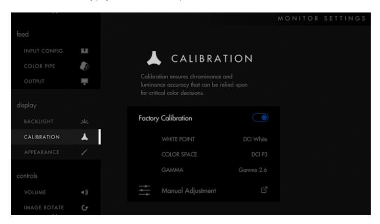
After clicking through the introduction, you will choose your calibration target. For non-HDR monitors, SDR - REC709 will be the recommended calibration. Select your calibration target and in the next screen, select Accept Calibration Target.
