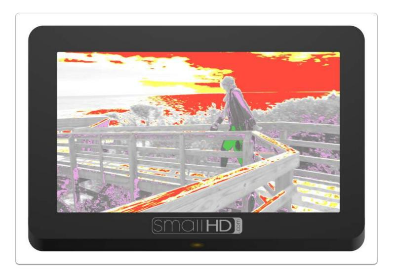
Exposure Assist is a great overall balance of utility and ease of use and can benefit most shooting scenarios. It allows 'painting' the image depending on the intensity of a pixel's luma value. For example you could set 97% IRE and up to turn bright red as an overexposure warning while creating a scale to turn green when a face is exposed properly at 55%, etc. (& anything else you wish to plot to any points on the range). Click to learn more about Exposure Assist.
