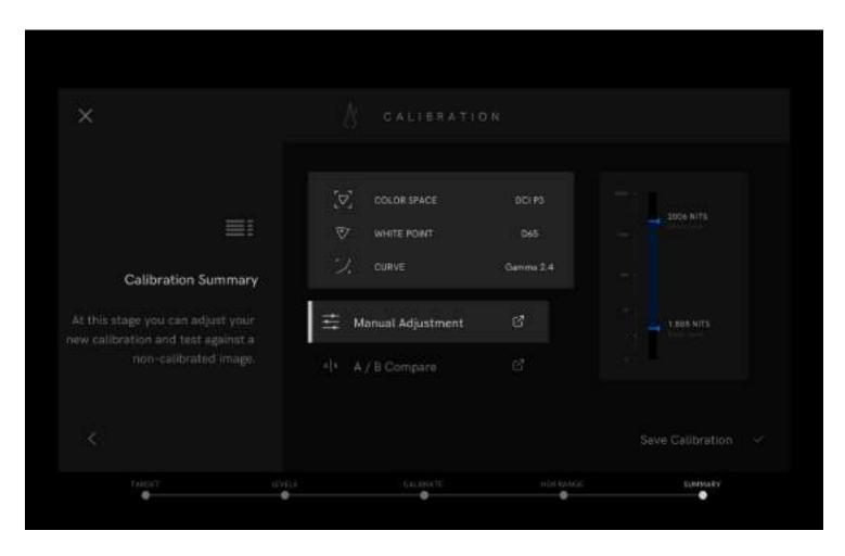
9. Your new calibration profile will automatically be applied and listed as **Custom Calibration** in the Calibration settings. You can toggle between **Custom Calibration** and **Factory Calibration** at any time.
