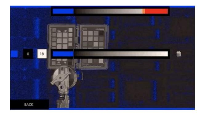
Set the **MIN** to **0** and adjust the **MAX** value to the point where color starts being introduced - You can customize this value until the **noise level** is acceptable to you (anything that gets painted blue is considered 'clipped', so increase the **MAX** to 'clip' more of the noise).
