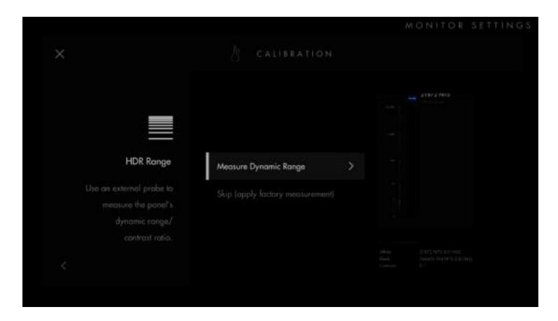
You will be presented with a Calibration Summary screen. Here you can use Manual Adjustment to tweak the calibration, as well as compare a before and after with A/B Compare. Select Save Calibration to save your settings.
