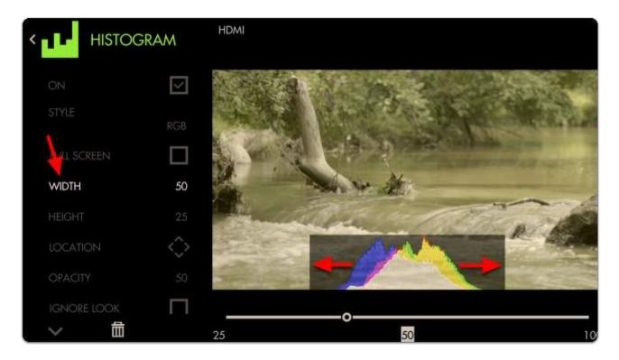
With the addition of RGB data, we can tell that our image has a warm cast toward the brighter end (yellow area) and a cooler cast in the shadows (blue area).
